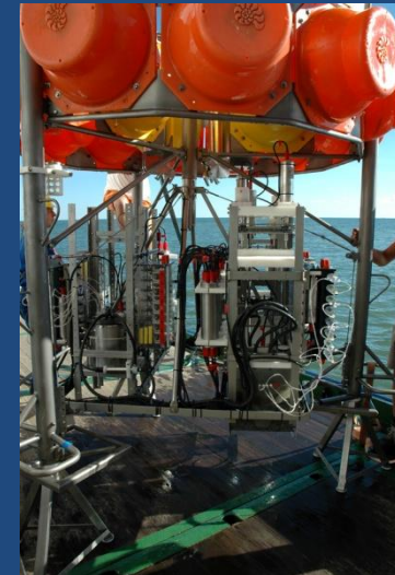
BIGO Biogeochemical Observatory Sommer et al., 2008
